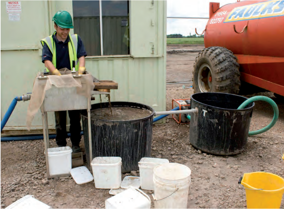
Fig 3 Flotation tank in use on the site of a Roman town along the A46. Practical constraints meant that a recycling system was developed for the on-site processing of whole earth samples. This made it possible to give rapid feedback to the excavation team (photo by J P Huntley).
