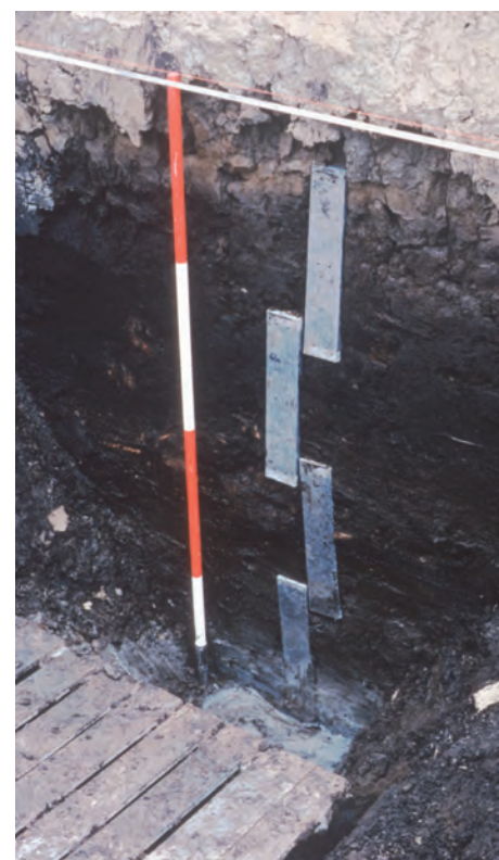
Fig 8 Glastonbury Relief Road: monolith tins in peat deposits overlying estuarine silty clays. Note the overlapping tins, which enable researchers to take samples from undisturbed positions throughout the length of the sequence. The monoliths were sampled for pollen and diatoms. Additional specialist samples from the same deposits were analysed for insects, macroscopic plant remains and foraminifera (photo by V Straker).
