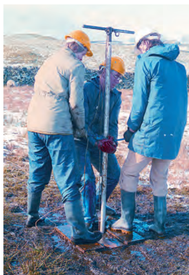
Fig 6 Using a modified Livingstone piston corer in kettle hole deposits on the A66 at Stainmore, County Durham (photo by J P Huntley).
