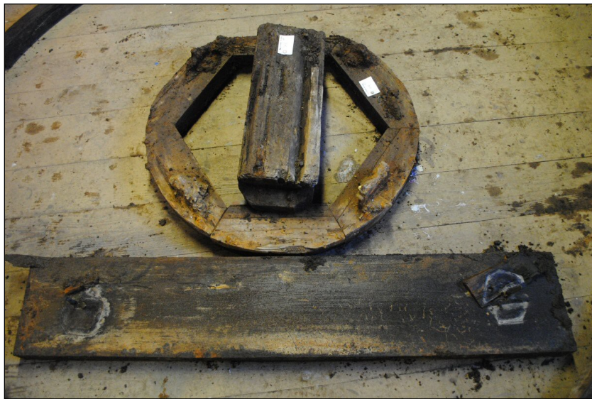
Illus. 26: Components of the inner ring of Buddle 1 following their removal.
