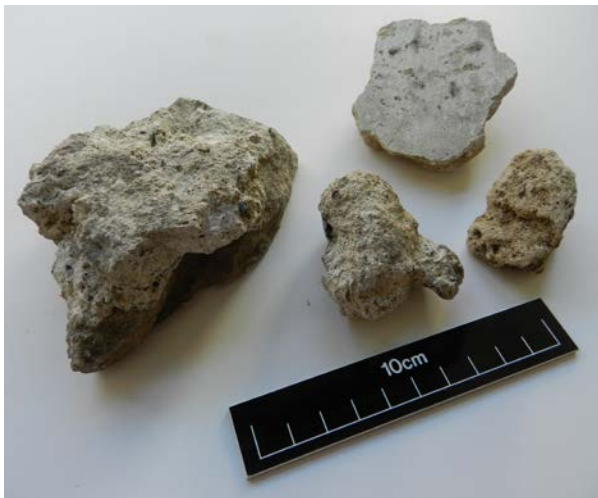
Plate 32 Building debris – from the back-fill of footing cut [8015] - SF859 and SF855; mortars and plasters of varying date; the yellowish pieces are likely to be medieval
